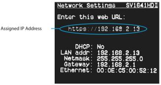
The initial screen will display the IP address assigned by your existing DHCP server (if present on your network). If no DHCP server is detected, a factory assigned IP address will be displayed in its place (10.0.0.15 by default). Please make note of the assigned IP address, as you will need to enter it into your web browser to access the Web Interface.
